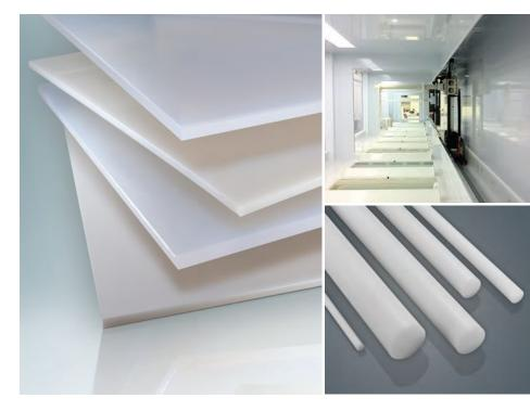
SIMONA<sup>®</sup> developed two grades of PVDF (polyvinylidene fluoride) sheet for diverse chemical process and semicon wet bench equipment. PVDF 740 Sheet offers higher stiffness and temperature resistance. PVDF-C 2850 copolymer sheet has more impact resistance and flexibility. Both perform well in many chemical environments, and are exceptionally resistant to concentrated acids and ultra-pure water (UPW) even at elevated temperatures.
